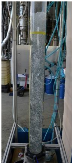
Smaller Cold Flow Model (100 mm inner diameter Ø)
